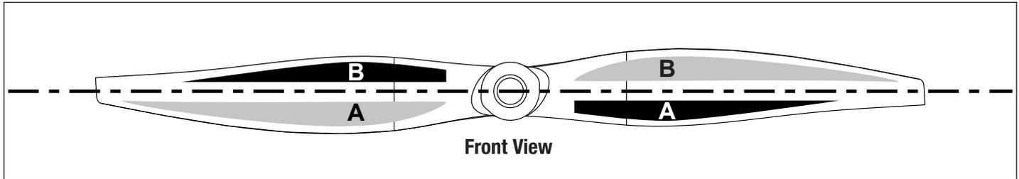
1. Remove the propeller from the aircraft then install the propeller on the balancer shaft. Make sure the propeller turns freely on the balancer shaft.
